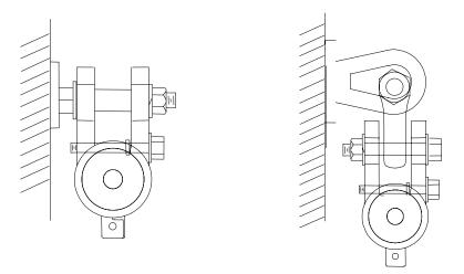
Figure 2 – Tangent Supports, Fixed (left) and Suspension (right) Assemblies
