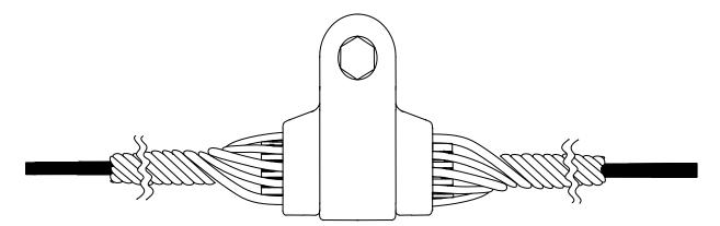
Figure 3 – Single Layer Heliformed Suspension Unit
